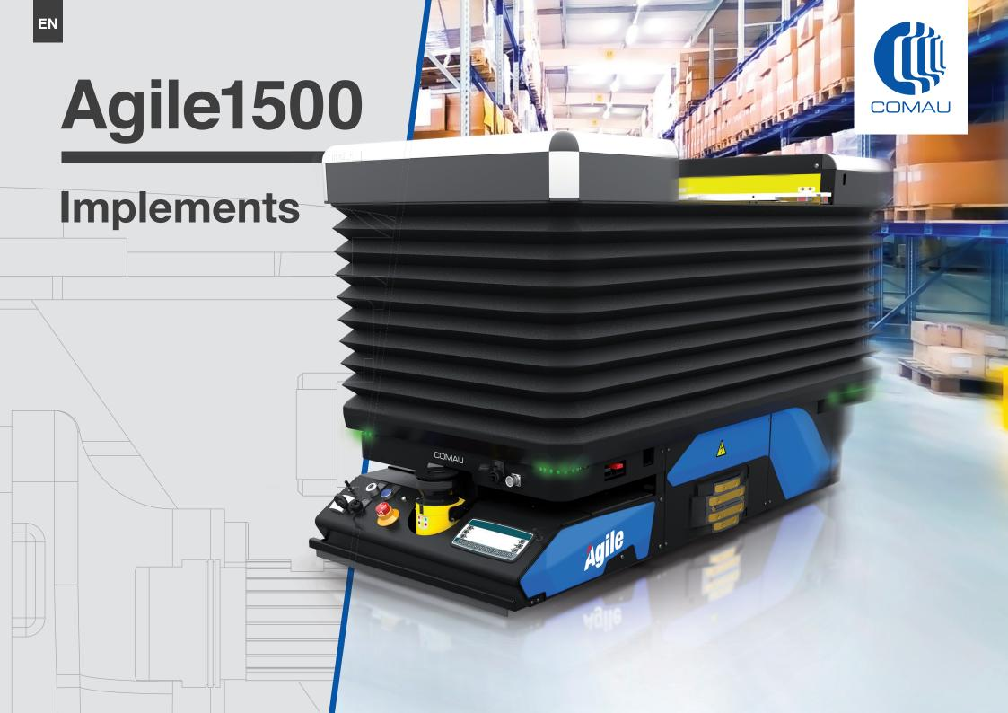
Comau presents the new automatic implements for Agile1500: Lifter400, with integrated conveyor, and Lifter1200. These off-the-shelf enablers are fully integrated with the base vehicle, powered by its long-lasting lithium battery. They can be applied in manual and automatic assembly systems, improving the ergonomic conditions of logistic operations.
